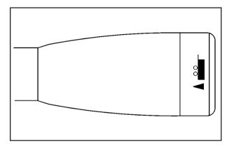
Your vehicle is equipped with a tow/haul mode. The button for this feature is located on the end of the column shift lever. You can use this feature to assist when towing or hauling a heavy load. See "Tow/Haul Mode" under *Towing a Trailer on page 4-53* for more information.
